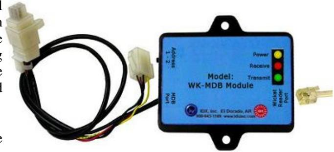
The WK-MDB Module is designed to provide the electrical and protocol interface between a vending machine controller (VMC) and a WR88 Wicket Reader. Its three diagnostic LED indicators provide visual operational information that may be helpful during installation and for troubleshooting problems. The enclosure dimensions are 3.0" L x 2.5" W x 1.0" H (76mm x 63mm x 25mm) and has integral mounting ears.
