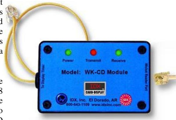
There is an RJ-11 telephone style connector on the right side of the enclosure to plug in the WR88 Wicket Reader. There is also an attached 16" RJ-11 telephone style cable assembly on the left hand side of the enclosure to plug directly into the Card-Display Protocol compatible display-timer.
